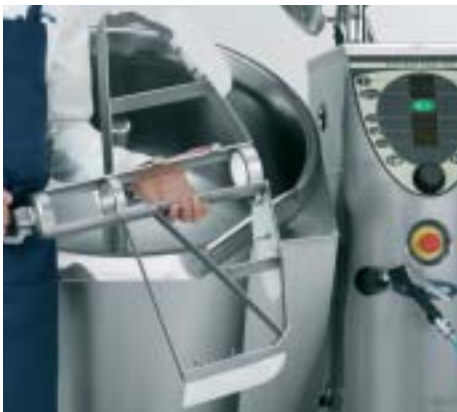
The only mixing tool with lift off scrapers for all kind of mixing. Light but strong, unique shape.
