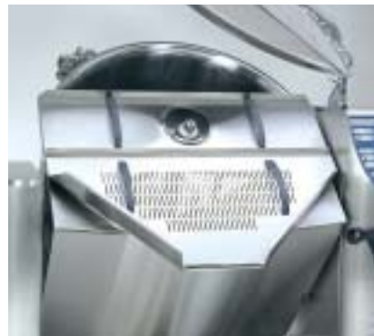
Two-part strainer plate (300-400 l). Additional part is used when necessary.
