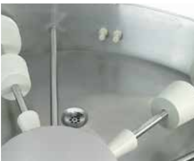
Drain in the bottom of the basin.
