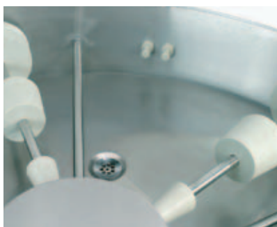
Drain in the bottom of the basin.
