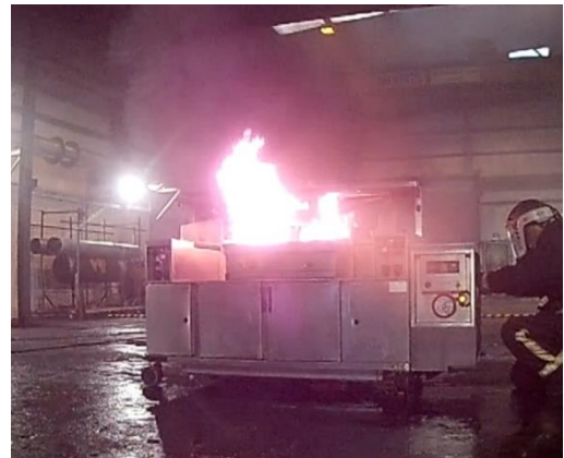
Fire as light bulb ruptures
