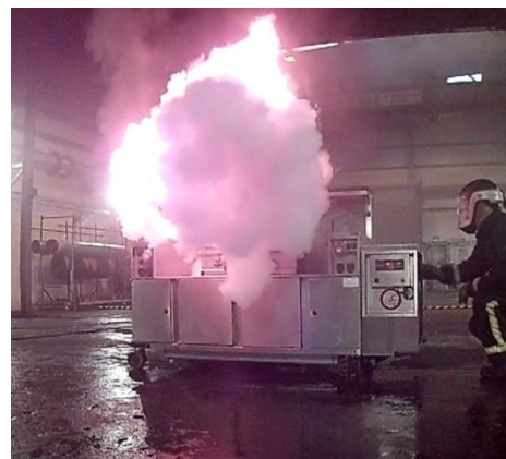
Immediately after activating suppression system
